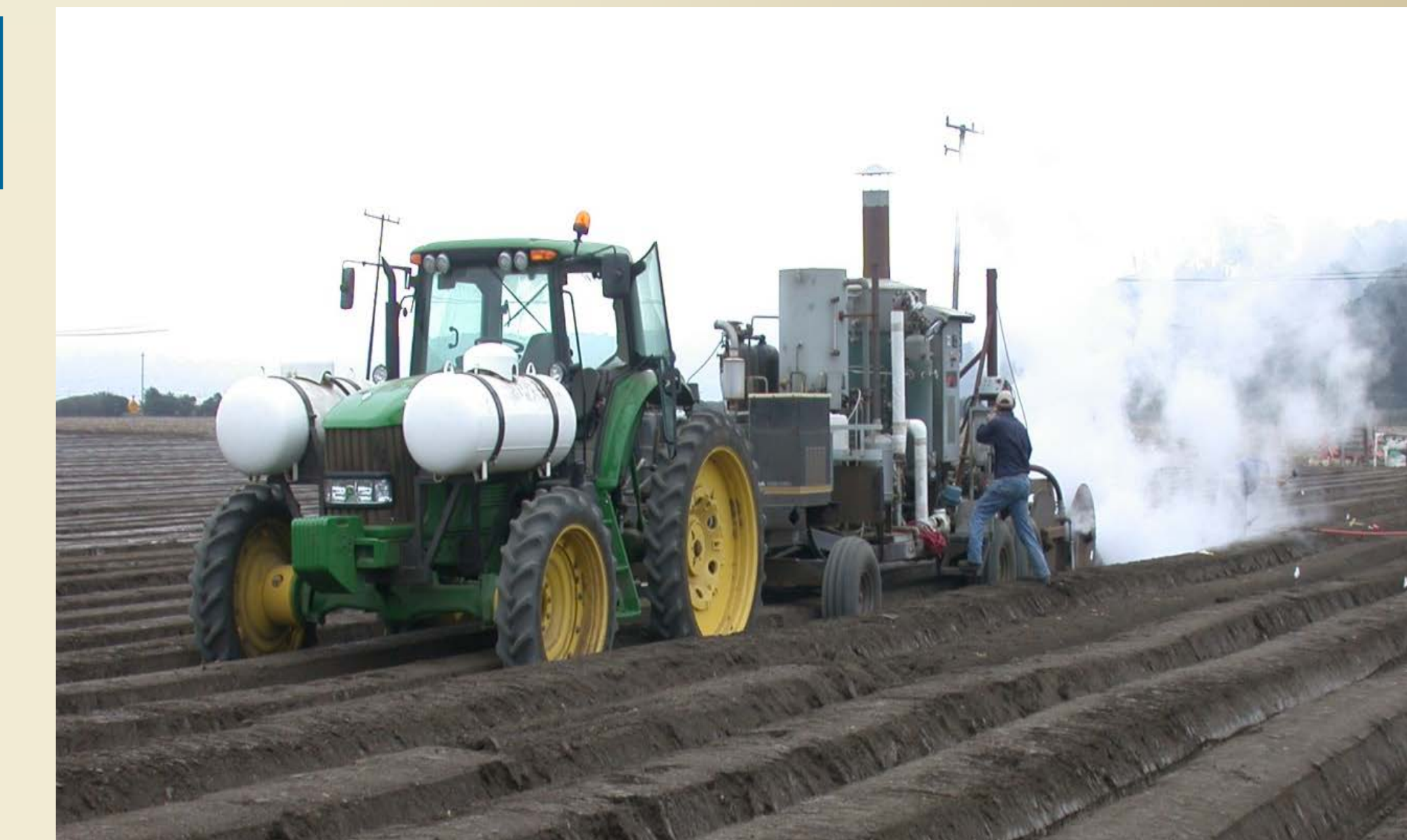
Tractor towed steam soil disinfestation machine. Proto Type, owned by Reiter Inc.. Able to disinfect shaped beds.
